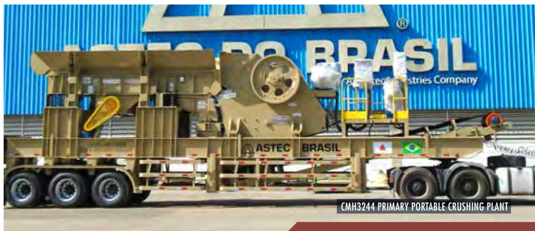
COMPLETE CRUSHING PLANT WITH H3244 HYDRA JAW CRUSHER, VGF 48X16 FEEDER AND 5' X 14' DD VIBRO KING SCREEN
