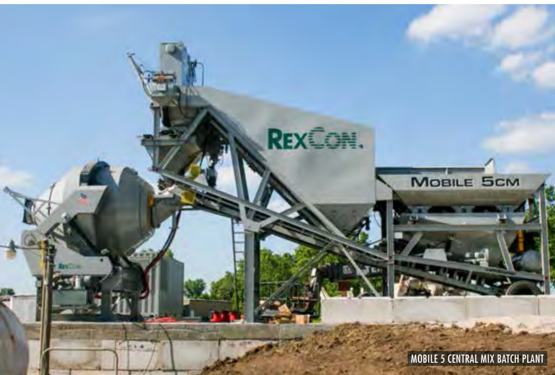
MODEL S BATCH PLANT WITH HORIZONTAL MIXER
