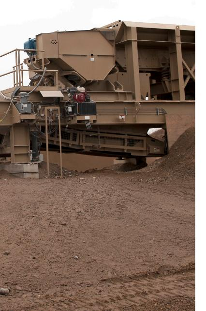
The 2056 Pioneer Jaw Crusher is a newly-designed, more compact model that features a 20" by 56" jaw crusher that is ideal for all crushing applications. The small gap provides an excellent nip angle at a tight closed-side-setting, making it a perfect fit for applications where material is minus-16", according to Tim Harms, product manager for Kolberg-Pioneer.
