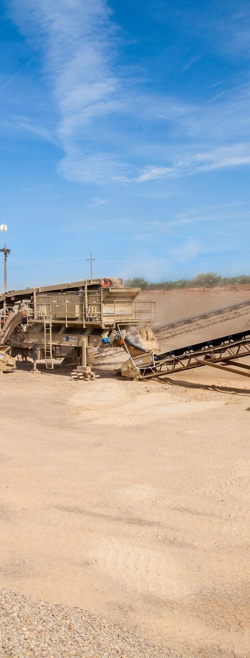
Harvey uses the GT205S to process concrete rock and hot-mix material. By utilizing three screen decks, he is able to make A4 rock, a size of material the company previously had to discard. Now, Big Creek Sand and Gravel is able to avoid wasting material and can offer more products to its customers, he said.
