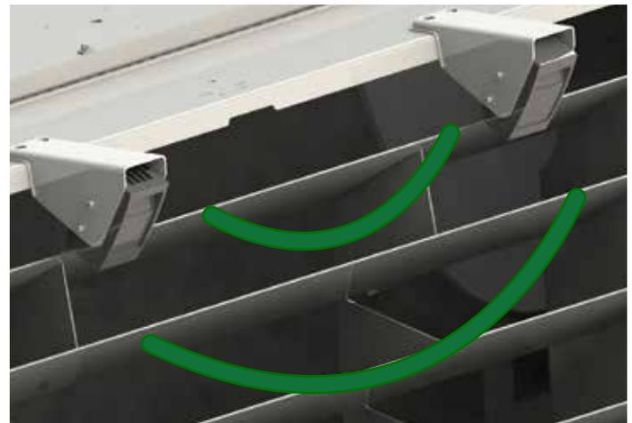
Sensors located on the back of the machine detect objects or people.
