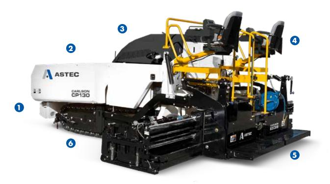
The single-piece cold-rolled steel frame provides heavy-duty structural support. All wear components and add-ons are bolted to the frame, making the CP130 fully-rebuildable for longer life cycle.
