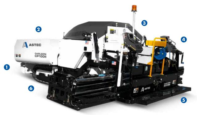
The single-piece, cold-rolled steel frame provides heavy-duty structural support. All wear components and add-ons are bolted to the frame, making the CP100 II fully-rebuildable for longer life.
