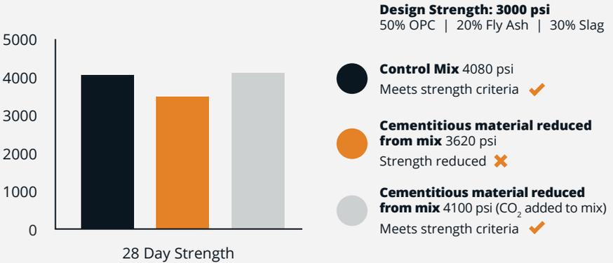
**Conclusion:** Adding CO<sub>2</sub> using CarbonCure enables concrete producers to remove their cementitious content and maintain compressive strength requirements.
