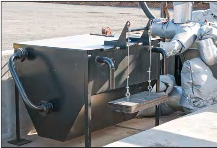
The hot box re-melts buckets of solidified asphalt that have been collected from samples used for testing. It has hot oil heating coils in its bottom and sides.
