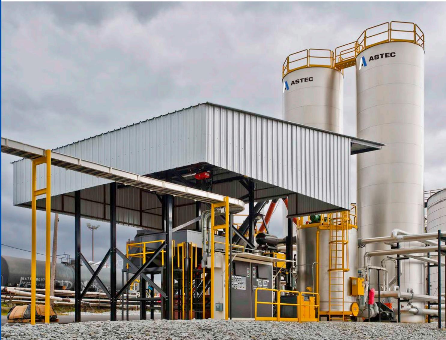
Astec provides equipment and services to build polymer blending systems. We were an early pioneer in producing systems to blend polymer with asphalt cement to make PMAC (Polymer Modified Asphalt Cement). PMAC is used as a binder in HMA (Hot Mix Asphalt). PMAC is also used to make asphalt roofing shingles to increase their life.
