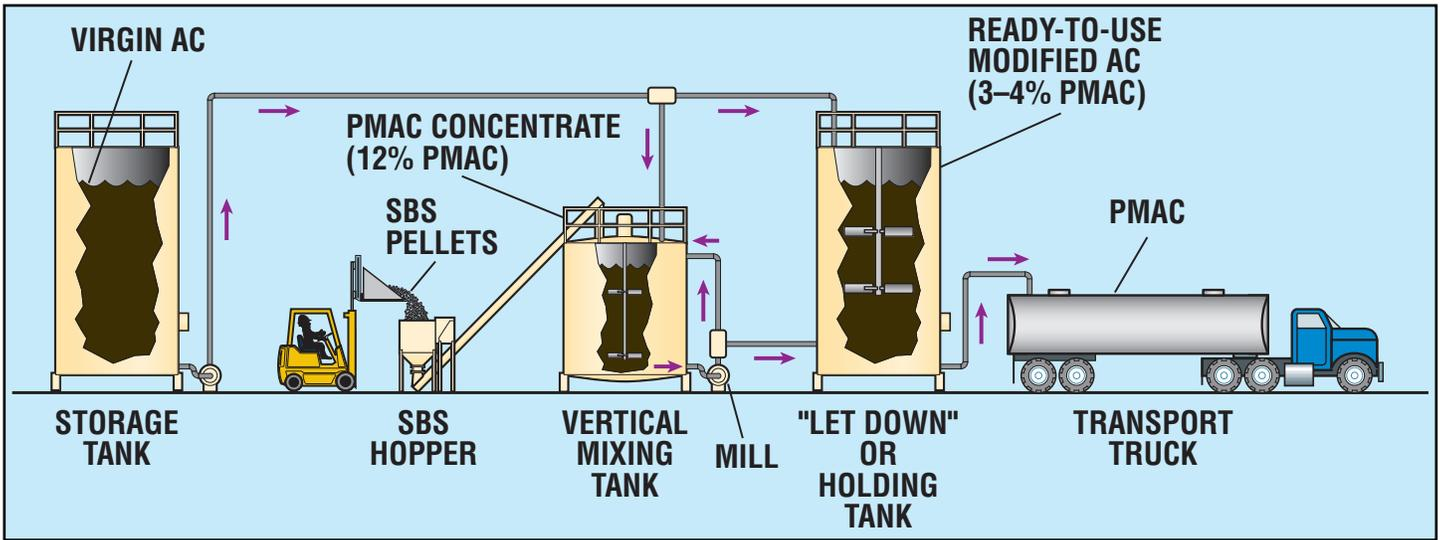
Typical Astec system for blending AC with SBS. Most systems have two vertical mixing tanks.
