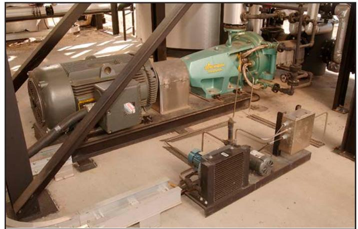
A Siefer mill is used to shear the polymer pellets into smaller pieces as they make multiple passes through the mill.
