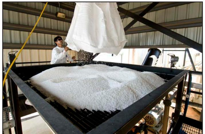
Here is a popular way to load polymers into the hopper of the blending system. The bags of polymer are hoisted over the hopper and untied so the material fills the hopper.
