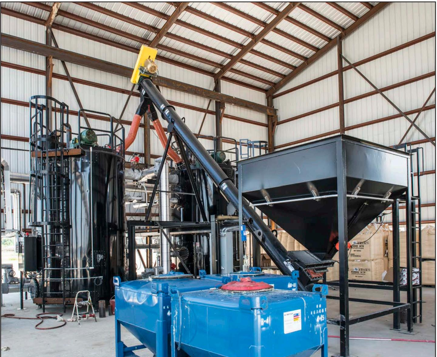
Polymer pellets are augured into the two mixing tanks shown in the background from the hopper on the right side of the photo. A "pant leg" chute allows the pellets to be diverted into either tank.
