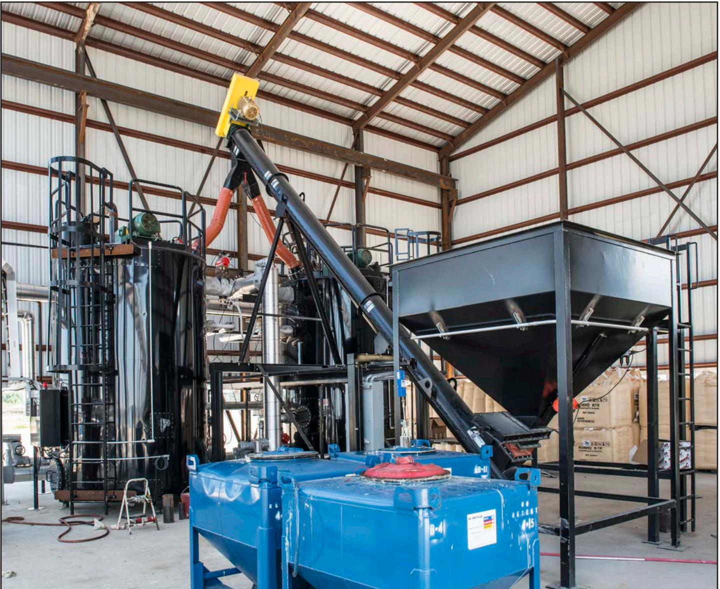
Polymer pellets are augured into the two mixing tanks shown in the background from the hopper on the right side of the photo. A "pants leg" chute allows the pellets to be diverted into either tank.
